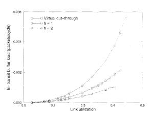
Fig. 8. In-transit packet load for virtual cut-through and hybrid switching.
