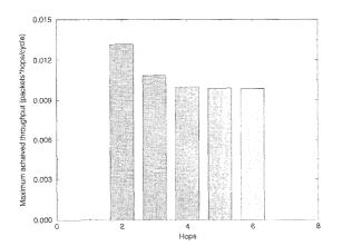
Fig. 4. Maximum throughput for wormhole switching under a hopuniform traffic load.
