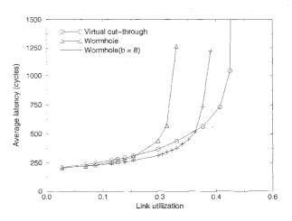
Fig. 5. Average packet latency for "buffered" wormhole.
