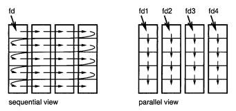
Fig. 2. A simple way to get a parallel view of a declustered file.
