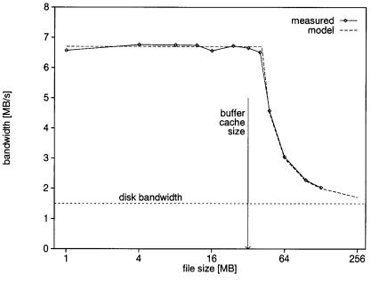
Fig. 11. Write bandwidth as a function of data set size.
