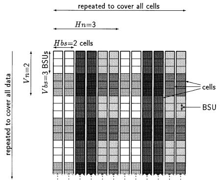
Fig. 3. The Vesta file-partitioning parameters. Subfiles are identified by different shades of gray.
