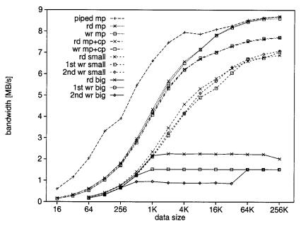
Fig. 10. Bandwidth as a function of data size, for message passing and Vesta.
