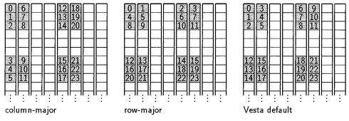
Fig. 4. Options for byte ordering with a subfile.
