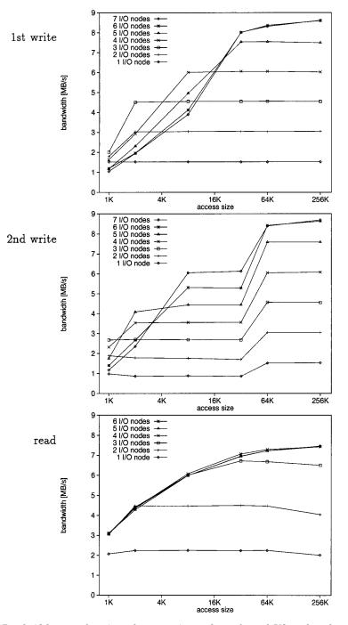
Fig. 12. Bandwidth as a function of access size and number of I/O nodes, for multiple asynchronous accesses.
