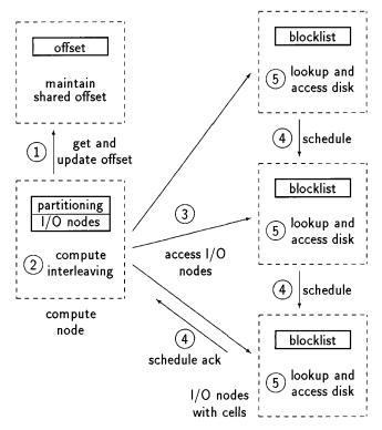
Fig. 8. The different stages of a file access. Steps 1 and 4 are optional.
