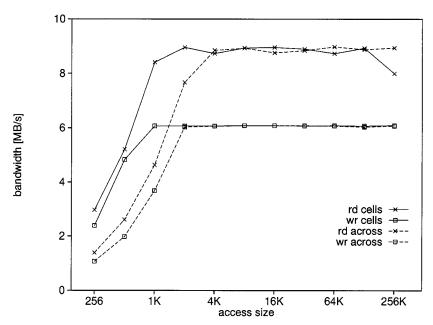
Fig. 16. Bandwidth as a function of access size for different partitioning schemes, with four compute nodes and four I/O nodes.
