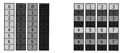
Fig. 15. Two ways to partition a Vesta file: Subfiles correspond to cells, or they are striped across cells.
