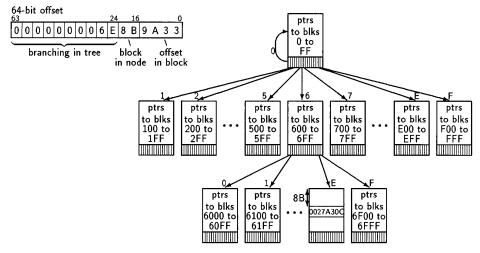
Fig. 9. Example of locating a data byte from its 64-bit offset. It turns out to be at offset 9A33 into logical block 0027A30C.
