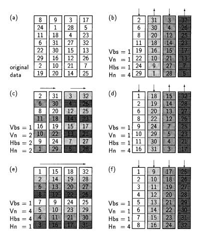
Fig. 6. Example of using subfiles to implement FastMeshSort on a file with four cells and eight records in each.
