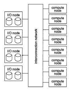
Fig. 1. Generic multicomputer architecture with parallel I/O.
