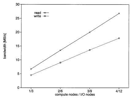
Fig. 13. Bandwidth as a function of system size, using a constant ratio of compute nodes to I/O nodes.
