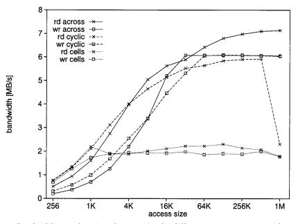
Fig. 14. Bandwidth as a function of access size for different access patterns, with a single compute node and four I/O nodes.
