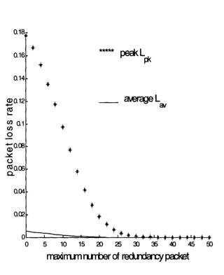
Figure 4. Packet loss rates versus the maximum number of redundancy packets for K = 32,  $\gamma_0 = 6$  dB, M = 50.
