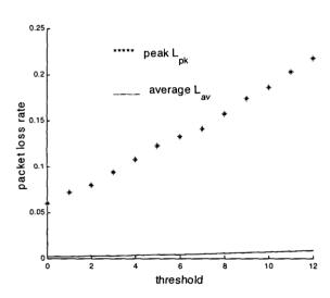
Figure 3. Packet loss rates versus SNR threshold given M = 50 and no redundancy packets.
