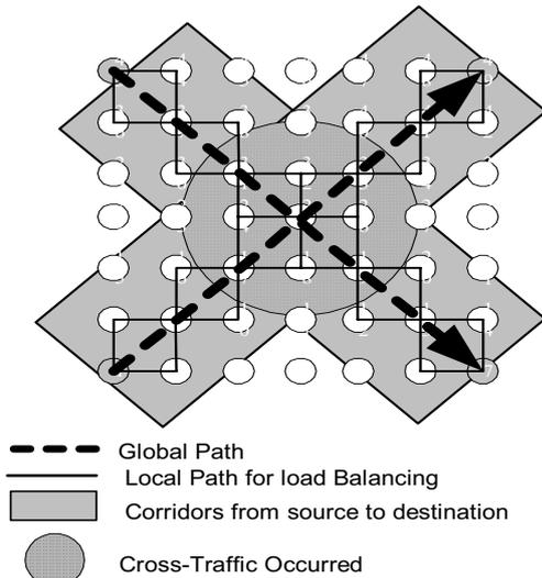
**Fig 3: Load Balancing Adaptive Zone Routing Protocol**
