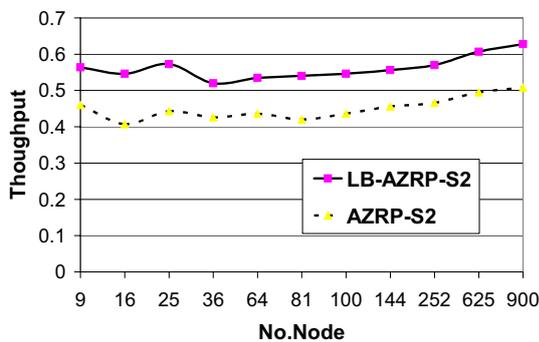
**FIG 7: Throughputs of AZRP and B-AZRP (Scene 2)**
