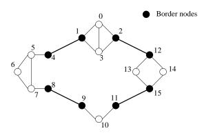
Fig. 4. A 2-level hierarchical network.
