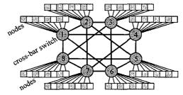
Fig. 10. Architecture of the T1 cluster computer interconnected by a high performance wormhole switch fabric.
